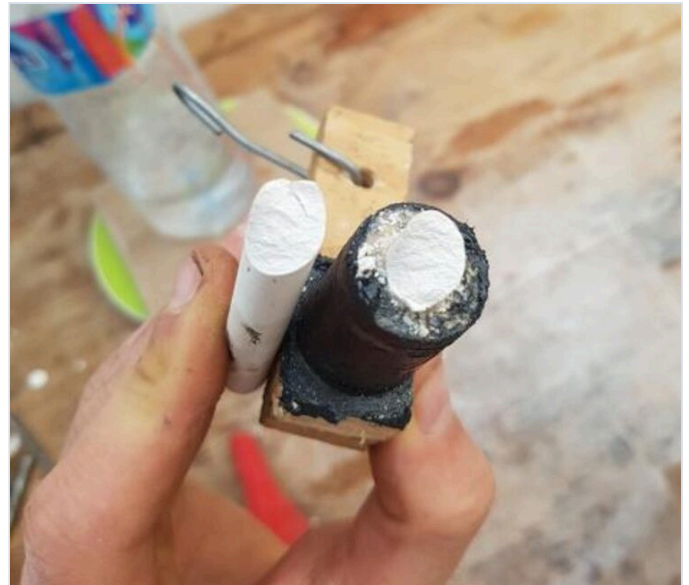
Characteristic helicoidal fracture from the torsion rig — evidence the load was correctly isolated.
